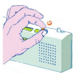
On the side of Olinda is the 'hardware API': seven bumps with sprung connectors carrying power, audio and control codes. New modules fit on with a clunk, and are held by embedded magnets. They also pass on the hardware API so modules can be daisy-chained together.
